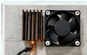
Cooling element (heat pipe, heat sink and fan)
