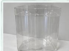
Acrylic reactor (2.5 L working volume)
