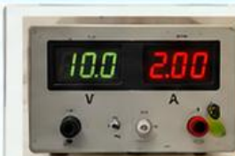
DC power supply (0–30 V, 0–10 A)
