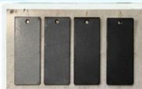
Interchangeable electrodes (Fe, Al, C, Pb)
